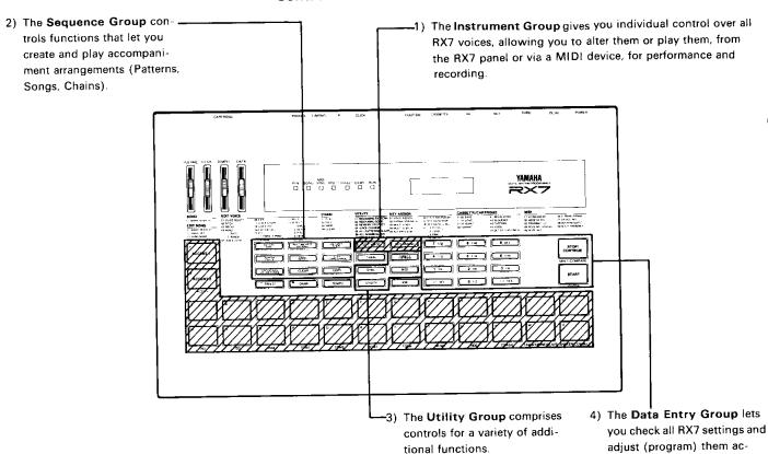
To keep the front panel compact, most keys have been given more than one function, so the order in which they are pressed is important. Always watch the messages on the LCD display for guidance. In many cases, dialog-type programming is possible, with the LCD asking you questions you can answer by pressing YES, NO or numeric keys.
