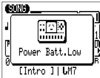
When this display appears, replace the batteries with a complete set of six new batteries. NEVER mix old and new batteries!
