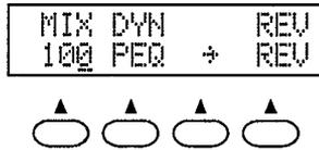
In this example the PEQ (Parametric Equalizer) effect of the DYN is combined with the REV (Reverb) effect of the REV group. The arrow between these parameters indicates that the normal serial connection is selected (DYN → REV). The DYN and REV parameters can be selected and other effects specified by pressing the corresponding function button and then using either the function button itself or the [▲] and [▼] keys.
