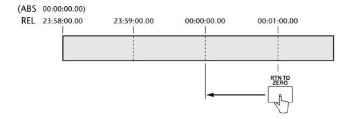
If the current project doesn't have a zero position, for example, the project starts at the absolute time of 01:00:00.00, the Return to Zero function locates the top of the project.
