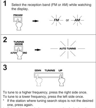
\* If the tuning search does not stop at the desired station (because the signals of the station are weak), change to the MANUAL TUNING method.
