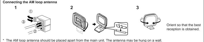
\* The AM loop antenna should be kept connected, even if an outdoor AM antenna is connected to this unit.
