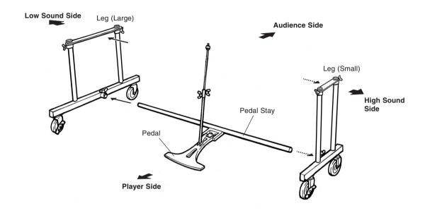
5 Connect the large leg and small leg with the pedal stay.
