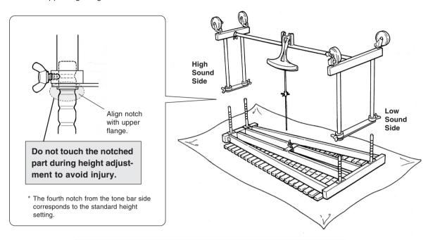
When a slide leg fixing bolt is tightened in between two notches, there is a danger of the slide leg slipping. Always make sure that the slide legs are held securely.
