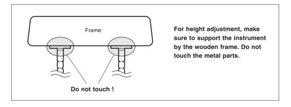
Lift the frame ends to the desired height and then securely tighten each slide leg fixing bolt, aligning it with the corresponding notch of the slide leg. Bolt and notch are aligned when the next higher notch is flush with the upper leg flange. (Refer to step  $\boxed{7}$  on page 24.)
