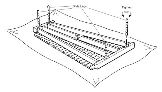
4 Place the large leg, small leg and pedal stay so that after assembly each part will be positioned as illustrated.
