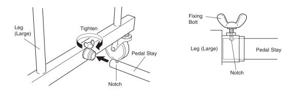
6 Connect the other end of the pedal stay with the small leg in the same way.
