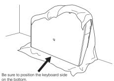
Spread a large soft cloth, such as a blanket, on the floor. Place the unit on the cloth with the key cover closed and the keyboard side on the bottom and lean the unit against the wall so that the unit will not fall or slip.
