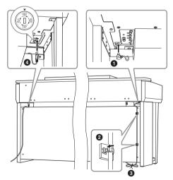
For models that feature a voltage selector: Set the voltage selector to an appropriate voltage.
