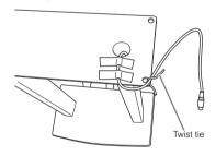
② Align the cord with the groove on the unit, and attach the pedal box using four screws.
