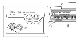
2 Connect the microphone to the [MIC./LINE IN] jack.
