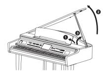
For the longer stay, use the inner recess, and for the shorter stay, use the outer recess to support the lid.
