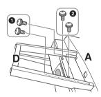
Fix unit D to the speaker box of unit A using two short screws (5 x 18 mm).
