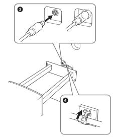
4 Attach the cord holder on the unit as shown in the illustration below, then use the cord holder to affix the pedal cord.
