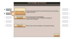
**5** Press the [B] button to select "LAN cable," then press the [G] button to proceed to "NEXT."
