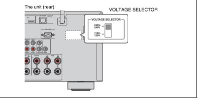
After all the connections are complete, connect the supplied power cable to the unit and then to an AC wall outlet.
