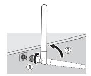
① Rotate the antenna clockwise.
