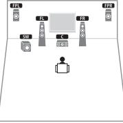
This speaker system uses the front presence speakers to produce a natural 3-dimensional sound field, and creates the virtual surround speakers using the front speakers to allow you to enjoy multi-channel surround sound (Virtual CINEMA DSP).
