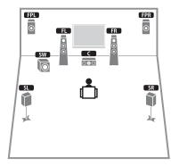
This speaker system uses the front presence speakers to produce a highly-natural 3-dimensional sound field, and is suited for enjoying 5.1-channel contents.
