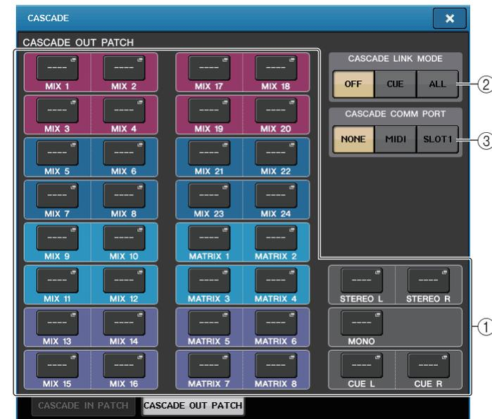
1. **Touches OUT PATCH (Assignation de sortie) (section CASCADE OUT PATCH)**
