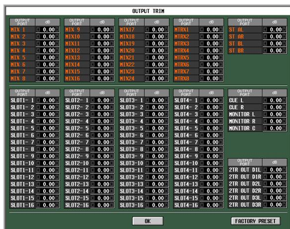
To adjust the gain, click the  $\uparrow$  /  $\downarrow$  buttons located at the left and right of each box to specify the gain of each output port in 0.01 dB units. If you want to reset all output ports to 0.00 dB, click the FACTORY PRESET button. Click the OK button to apply the settings.
