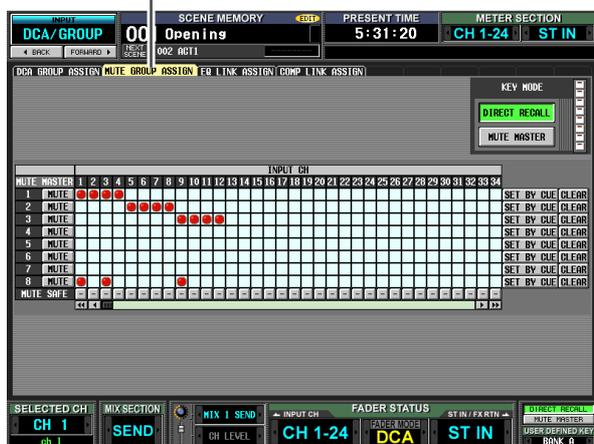
Except for the fact that these settings apply to input channels, the display and operations are the same as in the OUTPUT DCA/GROUP function MUTE GROUP ASSIGN screen. Refer to p.235.
