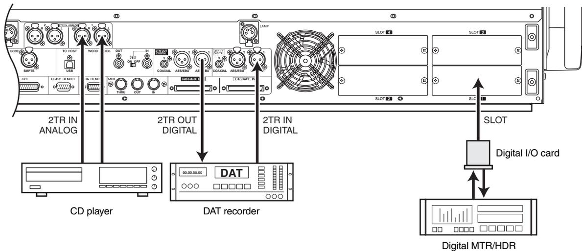
Use 2TR IN DIGITAL jacks 1–3 to connect digital sources such as CD players or DAT recorders. (To input analog output signals from a CD player or DAT recorder, use 2TR IN ANALOG jacks 1/2.)
