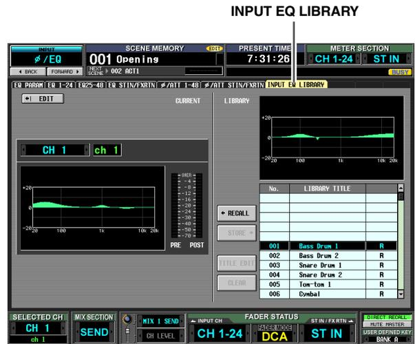
Except for the fact that these are EQ settings for the input channels, display and operations are the same as in the OUTPUT EQ function OUTPUT EQ LIBRARY screen. Refer to p.228.
