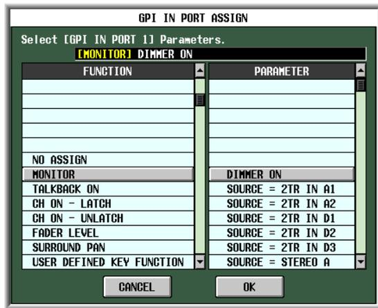
In the GPI IN PORT ASSIGN window you can select the PM5D function that will be controlled by each GPI IN port.
