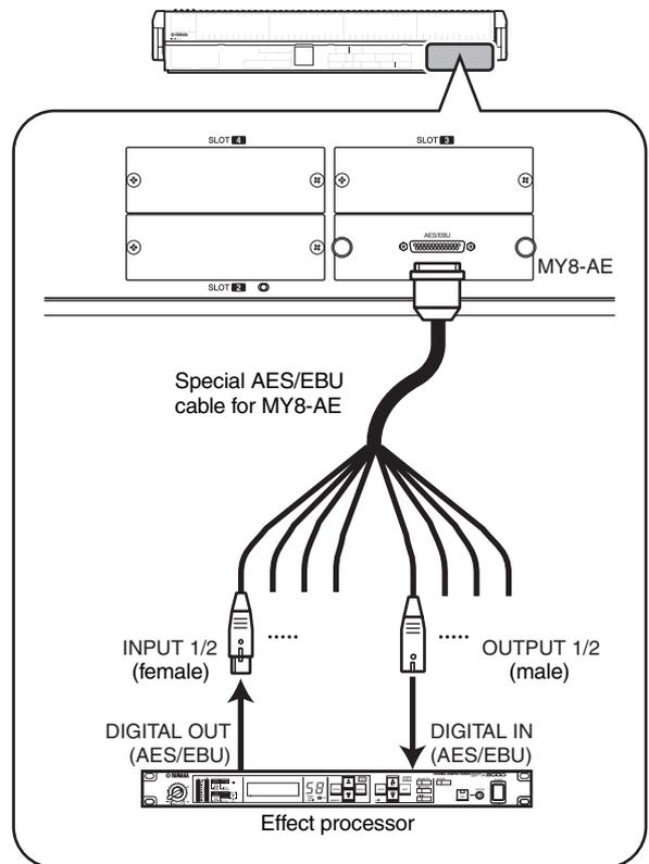
If you are inserting an external digital device via a digital I/O card as shown in “Insert connection example ③,” you will need to synchronize the word clock of the PM5D and the external device. Normally, we recommend that you set the external device as a word clock slave, and make it follow the PM5D’s word clock. (For details on how to set your device as a word clock slave, refer to its manual.)
