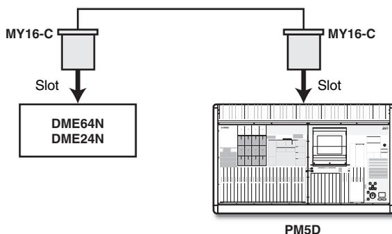
② **Bi-directional connection using the CASCADE IN/OUT connectors (DME64N only)**
