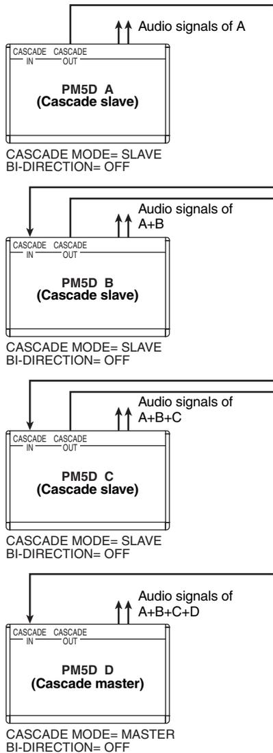
In this state, the SLAVE units will follow when you operate the MASTER unit. The final mix of all signals will be output from the PM5D that is connected last in the chain.
