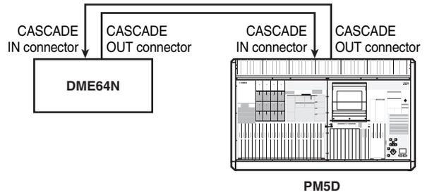
③ **Uni-directional connection using the CASCADE IN/OUT connectors — 1 (DME64N only)**
