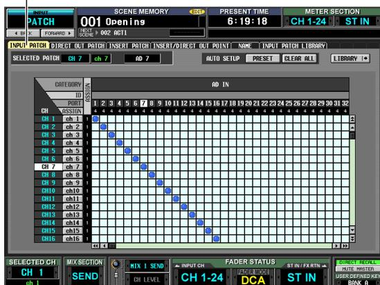
The INPUT PATCH screen is where you can patch (assign) input ports (rear panel input jacks or input channels of I/O cards) to input channels.
