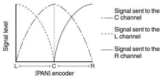
When the PAN knob ([PAN] encoder) is in the center position, the signal level of the CENTER channel will be at maximum, and no signal will be sent to the L/R channels.
