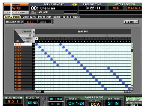
In the OUTPUT PATCH screen you can patch (assign) output channels to output ports. The horizontal direction of the screen shows the output ports (i.e., patch destinations), and the vertical direction of the screen shows the output channels (i.e., patch sources).
