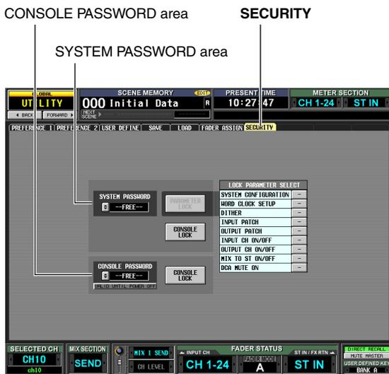
In this screen you can use the SYSTEM PASSWORD and CONSOLE PASSWORD fields located at the left to specify the passwords. (If no password has been specified, the corresponding box will indicate “--FREE--”.)
