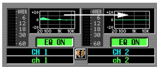
You can also copy EQ settings between the three screens EQ 1-24, EQ 25-48, and EQ STIN/FXRTN. First drag the mini-graph over the EQ 1-24, EQ 25-48, or EQ STIN/FXRTN tabs in the screen (the screen will switch). Then drag and drop the mini-graph onto the desired channel, and a window will appear, asking you to confirm the copy operation.
