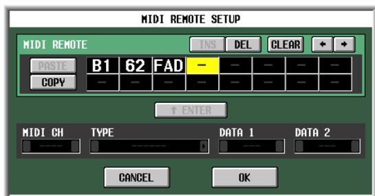
When you click a box in which a hexadecimal value has been input, the range of values that can be interpreted as a valid MIDI message (including that box) will turn red. The lower part of the screen shows the MIDI channel (MIDI CH), message type (TYPE), and data values (DATA 1, DATA 2) for this MIDI message, letting you verify that the appropriate MIDI message has been input.
