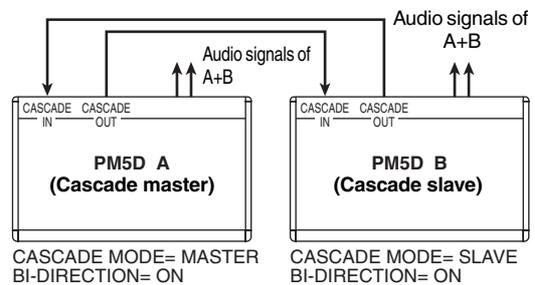
In this state, the SLAVE unit will follow when you operate the MASTER unit. The same mix will be output from both PM5D units.
