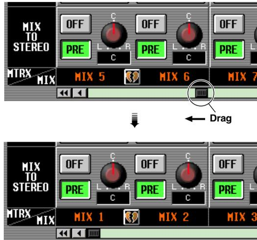
You can also scroll the screen by clicking the vacant portion of the scroll bar or the ◀/▶ buttons or ◀◀/▶▶ buttons located at the ends of the scroll bar.
