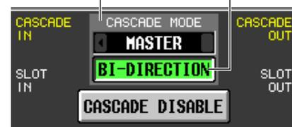
When multiple PM5D units are cascaded, the settings of the CASCADE MODE area specify whether the unit will operate as a cascade master (when "MASTER" is selected) or as a cascade slave (when "SLAVE" is selected).
