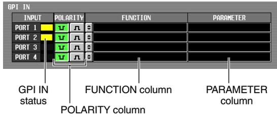
While the GPI screen is displayed, the GPI IN status column of the GPI IN area will show a yellow bar graph to indicate the approximate value of the voltage being input to each port. (If the bar is not shown, the voltage is grounded; if the bar is displayed all the way to the right edge, the voltage is at high level.)
