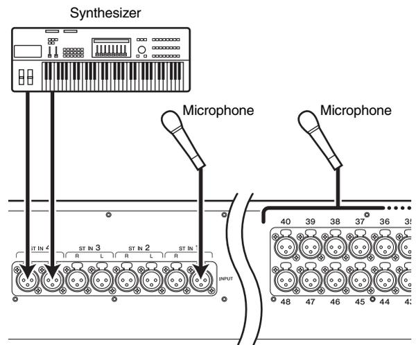
INPUT jacks 1–48 and ST IN jacks 1–4 can both be used to connect microphones or line-level devices.
