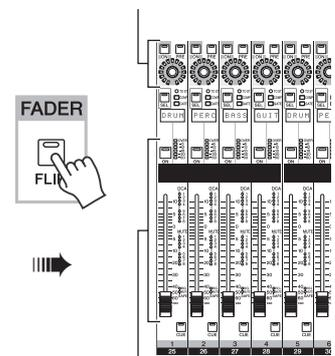
Control the send level and on/off status of the signal sent from the channel to the MIX buses
