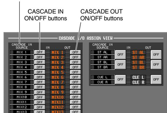
The **CASCADE IN** and **CASCADE OUT ON/OFF** buttons specify whether signals of each bus will be transmitted to or received from the cascade-connected external device. These settings are made independently for each bus; **MIX** buses 1–24, **STEREO A** bus L/R, **STEREO B** bus L/R, and **CUE** bus L/R.
