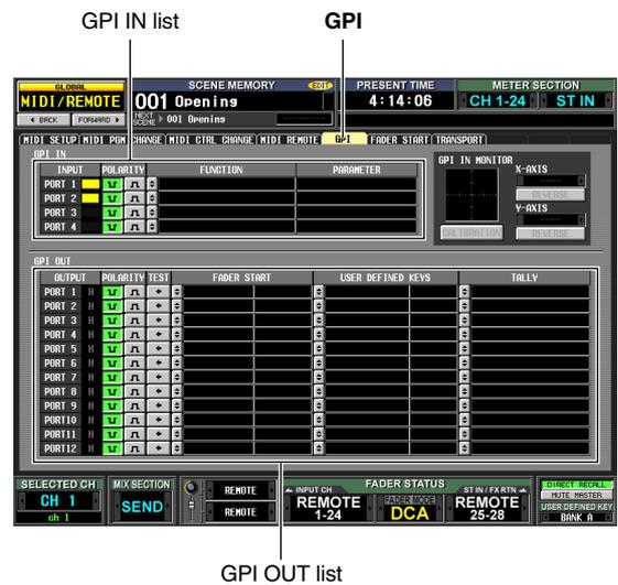
In this screen, the upper list is used to make GPI IN settings and the lower list is used to make GPI OUT settings.
