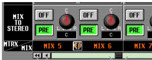
Click these buttons to move the scroll bar box step-wise in the direction indicated. Clicking the ◀◀/▶▶ buttons will move in larger steps than clicking the ◀/▶ buttons.
