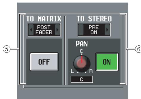
⑤ TO MATRIX (only for MIX channels and STEREO A/B channels)
