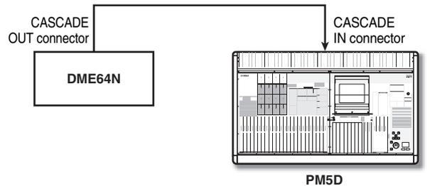
④ **Uni-directional connection using the CASCADE IN/OUT connectors — 2 (DME64N only)**
