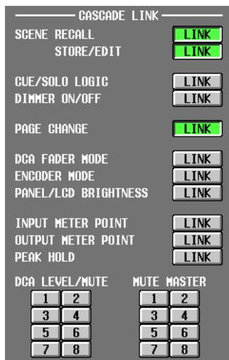
The settings of the **CASCADE LINK** area select the operations that will be linked when multiple **PM5D** units are cascade-connected. You can select the following items.
