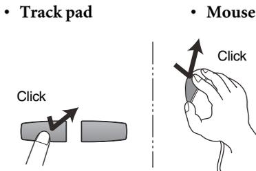
Using the CURSOR [◀]/[▶]/[▲]/[▼] keys of the data entry section to move the cursor to a desired parameter and then pressing the [ENTER] key is equivalent to clicking. If you are using a PS/2 keyboard, you can perform the same action using the arrow keys and the <Enter> key.
