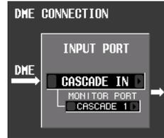
The types of port that can be selected here will depend on the port that is currently selected for cascade input (MIXER SETUP screen CASCADE IN PORT SELECT field), as follows.
