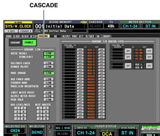
In this combination you can enable/disable buses used for transmission/reception in the cascade connection, and select the operations that will be linked when multiple PM5D units are cascade-connected.
