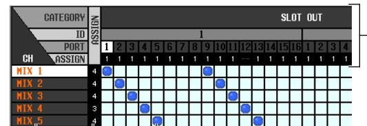
To patch an output port to an output channel, click this grid to display a “●” symbol.
