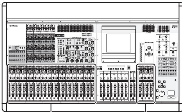
To each controller you can assign a MIDI message consisting of up to sixteen bytes of hexadecimal data. If desired, you can specify that a value within the message varies according to the movement of the controller.
