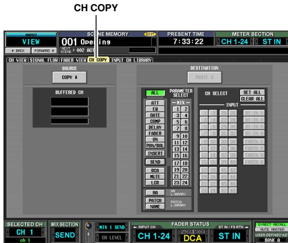
Except for the fact that these settings are for input channels, this is the same as the OUTPUT VIEW function CH COPY screen. Refer to p.249.
