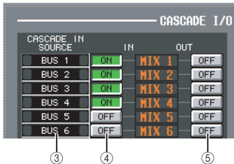
③ **CASCADE IN SOURCE (Cascade IN source I/O assignment view)**
