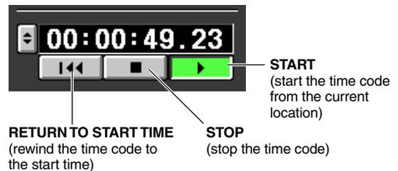
In addition, if INTERNAL is selected you can click the ▾ button to access the TIME CODE window, and specify the time code directly.
