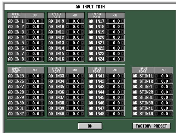
To adjust the gain, click the  $\uparrow$  /  $\downarrow$  buttons located at the left and right of each box to specify the gain of each input port in 0.1 dB units. If you want to restore all input ports to their factory settings, click the FACTORY PRESET button. Click the OK button to apply the settings.
