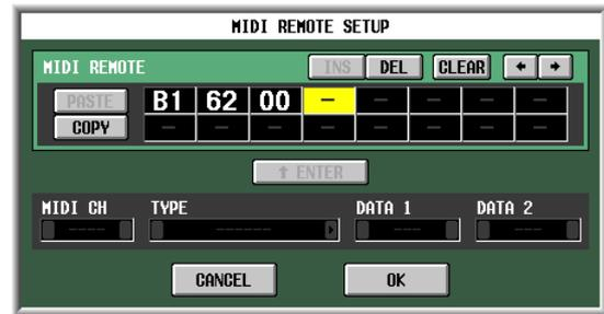
In this window you can input a message by clicking the desired input box to select it (the box will be highlighted) and turning the [DATA] encoder. You can use the [INC]/[DEC] keys to move the selected position. You can input the following values.
