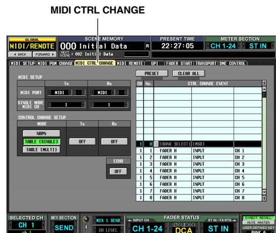
In the MIDI CTRL CHANGE screen you can select the port used to transmit/receive MIDI messages, and how control changes will be transmitted and received. If control change 1-119 is selected as the transmission/reception method, you can assign the desired event to each control number.
