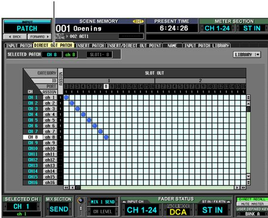
In this screen you can select the output port that will directly output the input signal of an input channel or ST IN channel. You can select the following output ports.
