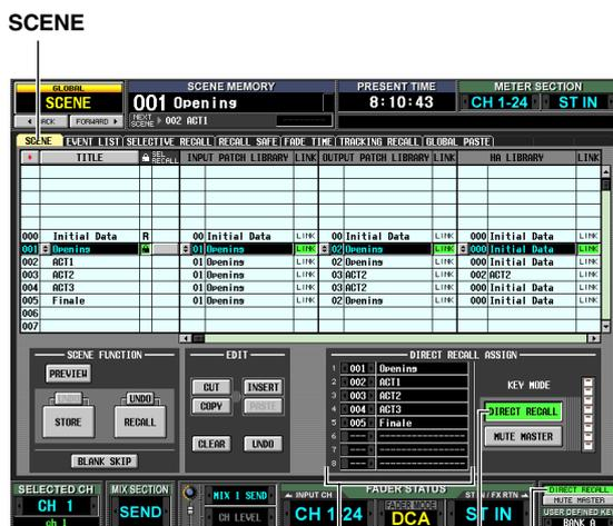
In the SCENE screen you can use the DIRECT RECALL ASSIGN list shown in the lower middle of the screen to assign scene numbers to the SCENE MEMORY [1]–[8] keys.
