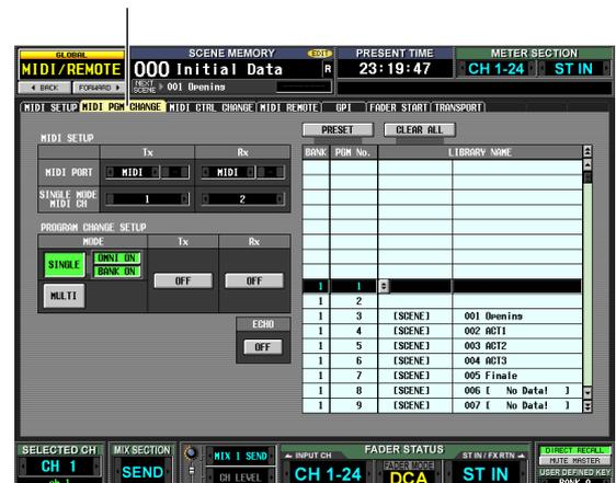
In the MIDI PGM CHANGE screen you can assign events to each program number, select the port at which MIDI messages will be transmitted and received, and select how program changes will be transmitted and received.
