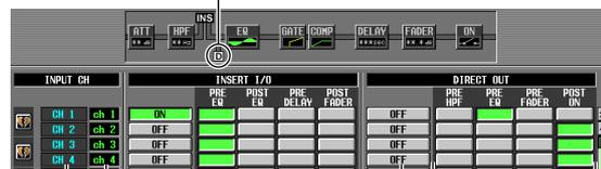
Switch direct out on/off for each channel.
