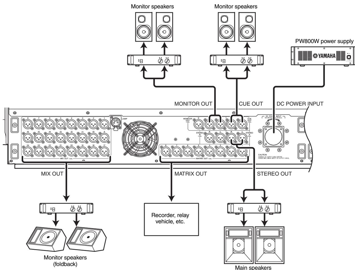
MIX OUT jacks 1–24, MATRIX OUT jacks 1–8, and STEREO OUT A/B jacks respectively output the signal from MIX channels 1–24, MATRIX channels 1–8, and the STEREO A/B channels.
