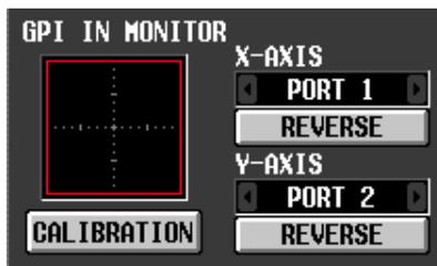
When you specify a GPI IN port, the voltage from that GPI IN port is indicated by a yellow ☉ symbol in the GPI IN monitor area. In this case, the horizontal position (X-axis) corresponds to the voltage of the GPI IN port selected in the X-AXIS field, and the vertical position (Y-axis) corresponds to the voltage of the GPI IN port selected in the Y-AXIS field.
