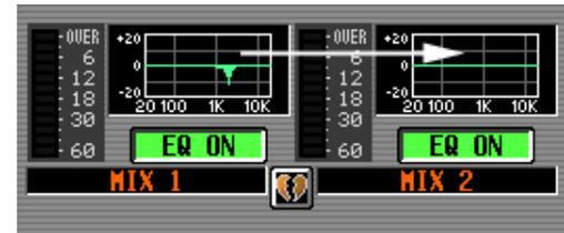
You can also copy EQ settings between the MIX 1-24 screen and the MATRIX/STEREO screen. First drag the mini-graph over the MIX 1-24 tab or MATRIX/STEREO tab in the screen (the screen will switch). Then drag and drop the mini-graph onto the desired channel, and a message will ask you to confirm the copy operation.
