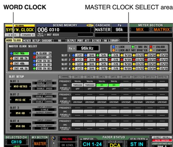
In this screen you can select the master clock, and check the input signal synchronization status for each slot or jack.
