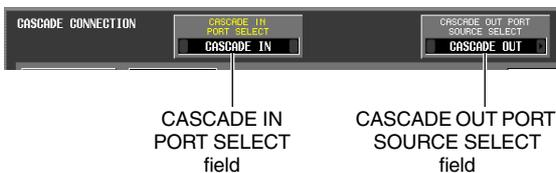
The CASCADE IN PORT SELECT and CASCADE OUT PORT SOURCE SELECT fields select the ports
