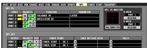
If the same port is specified for the FADER START parameter and the FADER STOP parameter, the GPI screen FADER START field will be assigned to the channel corresponding to that port (Fader Mode= FADER TALLY). (The opposite is also true.)
