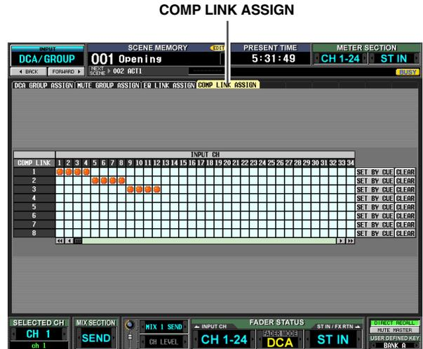
Except for the fact that these settings apply to input channels, the display and operations are the same as in the OUTPUT DCA/GROUP function COMP LINK ASSIGN screen. Refer to p.237.
