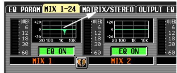
You can also copy settings between the eight-band EQ of a MIX channel or STEREO A/B channel and the four-band EQ of a MATRIX channel. In this case, only the LOWER four bands will be copied for MIX channels or STEREO A/B channels.
