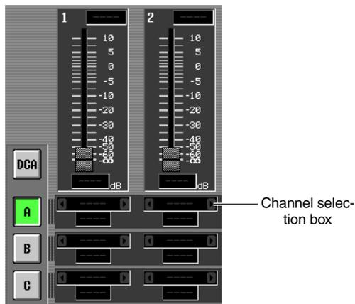
To select a channel, click the ◀ / ▶ buttons located at the left and right of each box. You can choose from the following channels.
