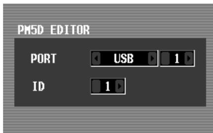
First use the PORT field to select the port that will be used to communicate with the computer. Click the / buttons located at the left and right of the left box to select the type of port, and press the [ENTER] key (or click inside the box) to finalize your selection. If you select USB or SLOT 1–4, use the box at the right to select a port number 1–8.
