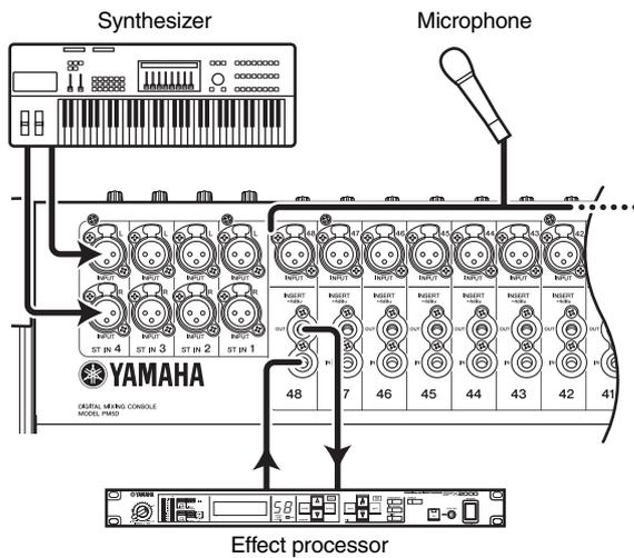
INPUT jacks 1–48 are used mainly to connect microphones or monaural line-level devices. ST IN jacks 1–4 are used mainly to connect stereo line-level devices.
