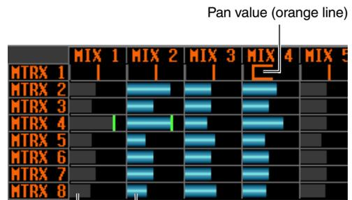
Channels for which the signal sent to the MATRIX bus is turned off (gray bar graph)      Channels for which the signal sent to the MATRIX bus is turned on (blue bar graph)
