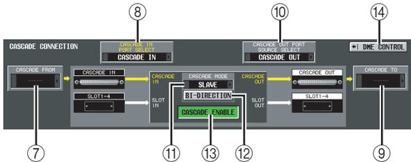
⑦ **CASCADE FROM (Source when cascade-connected)**
