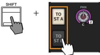
Set TO ST A and B for multiple channels
