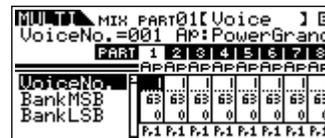
**NOTE** By selecting the BankMSB/BankLSB parameter with the cursor [^][v] buttons and using the data dial, you can call up the Voice Banks listed below.
