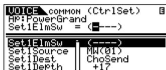
For example, in the instructions below, we'll control panning with an external Modulation wheel.
