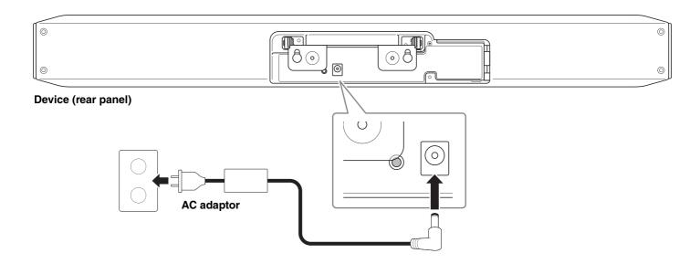
Connecting the AC adaptor automatically turns on the device.
