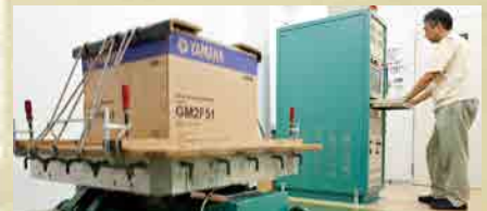
Vibration testing guarantees that no damage will occur during transportation and delivery around the world
