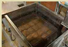
Shell sections are boiled and dried to test ply adhesion
