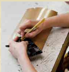
Cutting finishes to test adhesion
