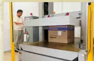
Compression testing simulates the pressures our packaging has to withstand when stacked
