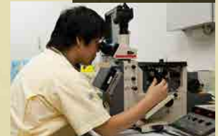
Microscopic examination of plating thickness and quality
