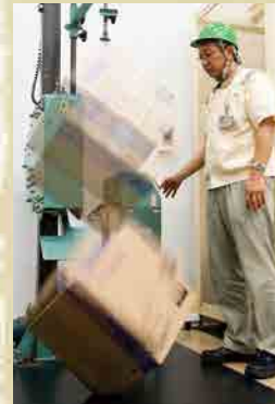
Drop tests ensure that our packaging will prevent damage to the instruments within under the harshest conditions
