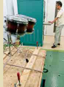
Vibration testing simulates tough playing conditions
