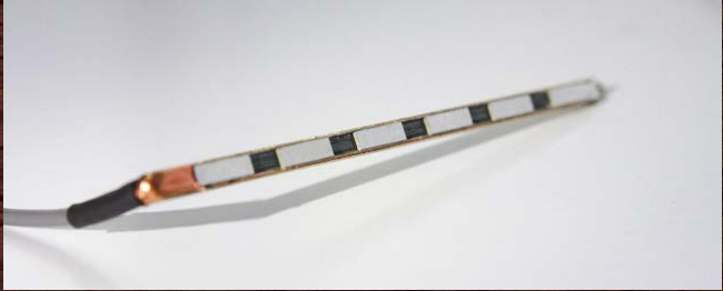
SRT Pickup Yamaha’s proprietary SRT pickup design uses individual elements for each string to give an ultra-clear, ultra-wide bandwidth signal with far better dynamic response and tonal accuracy than a regular, ribbon-type piezo pickup.
