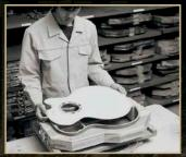
Gluing the Top to the Sides
