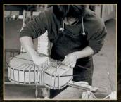
Attaching the Body Binding
