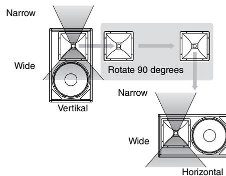
**NOTE** If you use the speaker as a floor monitor, change the horn dispersion so that the upward spread is wide and the downward spread is narrow, as shown in the diagram.
